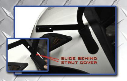
Attach brackets using retained hardware. Slide strut cover back down over bracket once attached.
