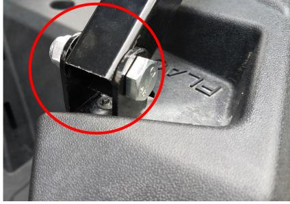
5. Once the Inner Support (F), Outer Support (H), and Extension Rail (K) are installed, it is time to position the assembly onto the vehicle. Remove the factory torx head bolt and place through the hole in the bottom of the lower Inner Support Tab (G). Reinstall torx head bolt back into the factory hole. Attach the Inner Support Tab (G) onto the lower hole of the Inner Support (F) using the supplied M10x45mm bolt and lock nut. See image above.
