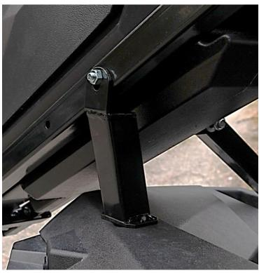
6. Next remove the factory torx head fastener from the recess of the bed side and install the Outer Support (H) as shown using M6x35mm flange head bolt. The Outer Support (H) sits on top of the recessed hole on the bed side so that it may be used on either the driver or passenger side of the vehicle. The rear of the R1 rack should now be supported by the bed so that the final clamp can be installed.
